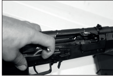
2) Make sure the chamber is empty
