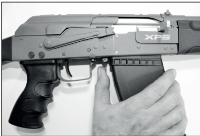
4) This is the position the shotgun should be in while loading or unloading
