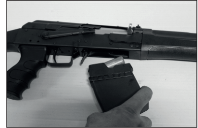
3) Load the magazine up to its capacity with correct caliber ammunition that complies with CIP standards.
