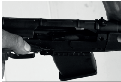
5) Pull the operating handle toward yourself and release it.
