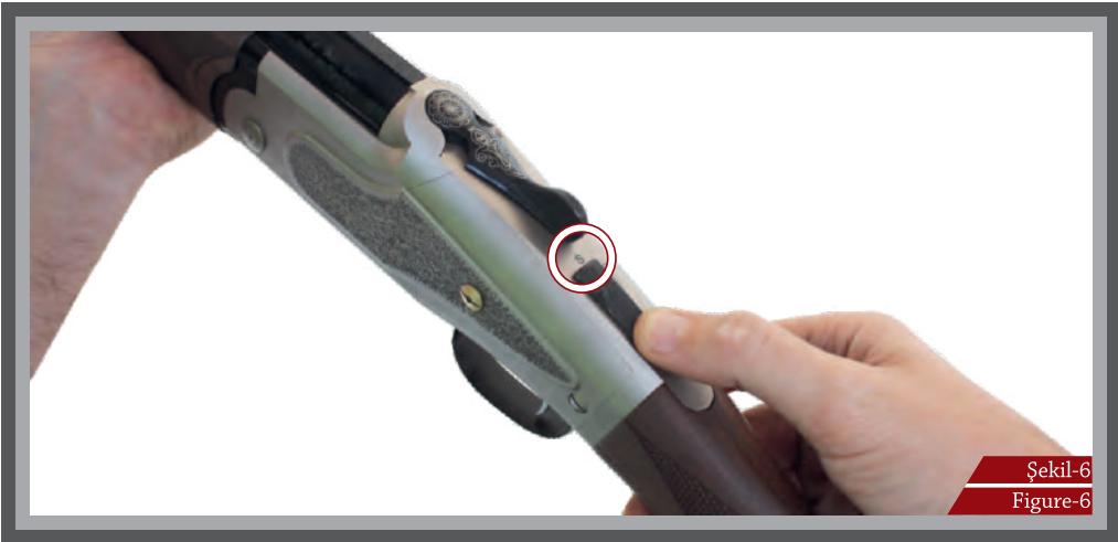
*The safety button is directly assembled into the trigger and it is located on the breech-top of the receiver. (Figure-6)
