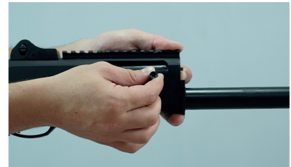
3 - Move back the mechanism and ensure that cocking lever comes to the middle of the mechanism bearing; then, pull out and remove the cocking lever. During this operation, hold the cocking-bar so that the spring doesn't push it forward
