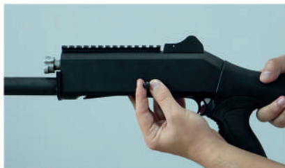
4 - Take out the trigger group anchor pin
