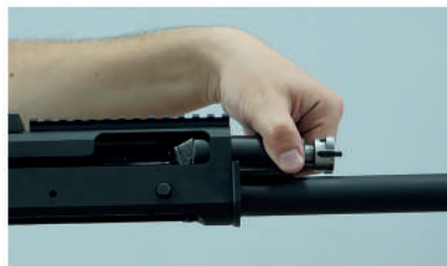
6 - After you remove the Trigger Group, the bolt assembly and action bar sleeve can be removed from the shotgun
