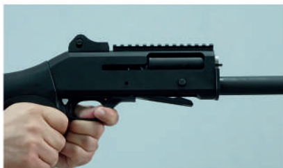
5 - Pull the trigger group and detach from the receiver
