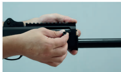
3 - Move back the mechanism and ensure that cocking lever comes to the middle of the mechanism bearing; then, pull out and remove the cocking lever. During this operation, hold the cocking-bar so that the spring doesn't push it forward
