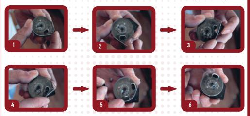
Once the glass cover hits are last point, prevent the pushing force of the spring and switch the Pellet to first bed(see picture 4). Once the first pellet prevents the rotation of the inner turret, move the glass cover on the contrary direction and fill the turret.
