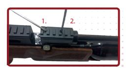
Dissamble the assemble screw of the receiver.(screw1)
