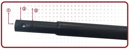
Barrel tightness o rings are three totatlly and 2 of them are outside ( ② ) ( ③ ) while 1 inside. ( ① ). Incase of deformation , please replace with the spare o rings that are available inside the packaging.
