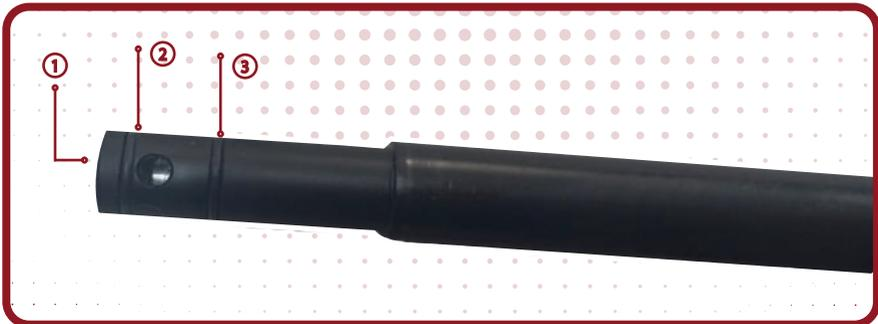
Barrel tightness o rings are three totatly and 2 of them are outside ( ② ) ( ③ ) while 1 inside. ( ① ). Incase of deformation , please replace with the spare o.rings that are available inside the packaging.
