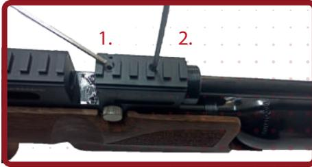
Dissamble the assemble screw of the receiver.(screw1)
